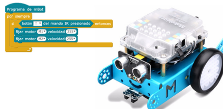
Figure 3.3: Mbot robot and programming example
